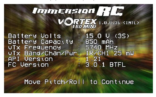
Moving the pitch/roll stick (right stick for mode 2'ers) will dismiss the menu.
